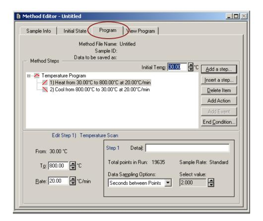
To change a step, click the line to highlight it. The temperature and rate at the bottom left corner are for the selected step. To add steps, you can either insert a step (above the highlighted line) or add a step (below the highlighted line). You can add temperature ramps or isothermal steps. To delete a step, just highlight the line and then click Delete Item.
