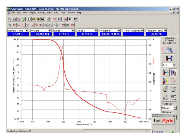
You can the type of data displayed using the Curves menu. The two most commonly used data are heat flow (endo) and weight.
