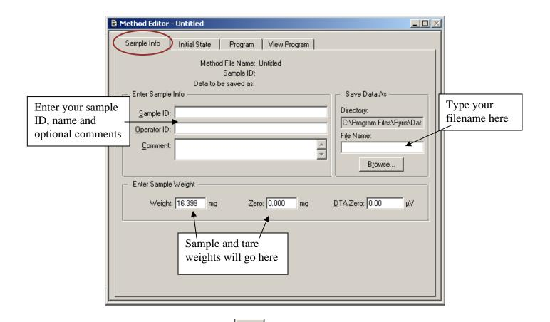
When you tare the pan, click on the icon on the right side of the screen. This will zero the weight, but will put a random, non-zero value in zero box on this Sample Info tab. You MUST change the zero to "0.000" in the box in order to continue!
